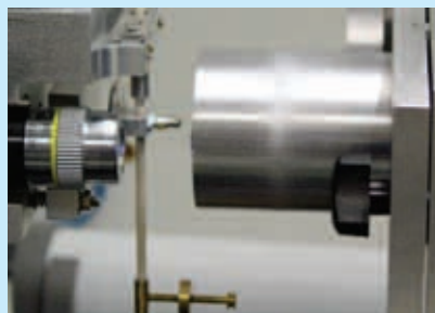
Loads of 0.1mN to 500mN are used to assess the micro-mechanical properties of samples using a diamond-tipped nano-indenter
