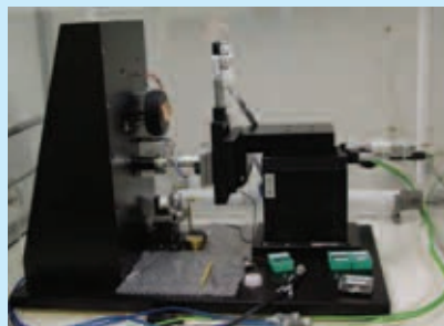
MicroMaterials NanoTest platform is contained within a temperature controlled environmental enclosure
